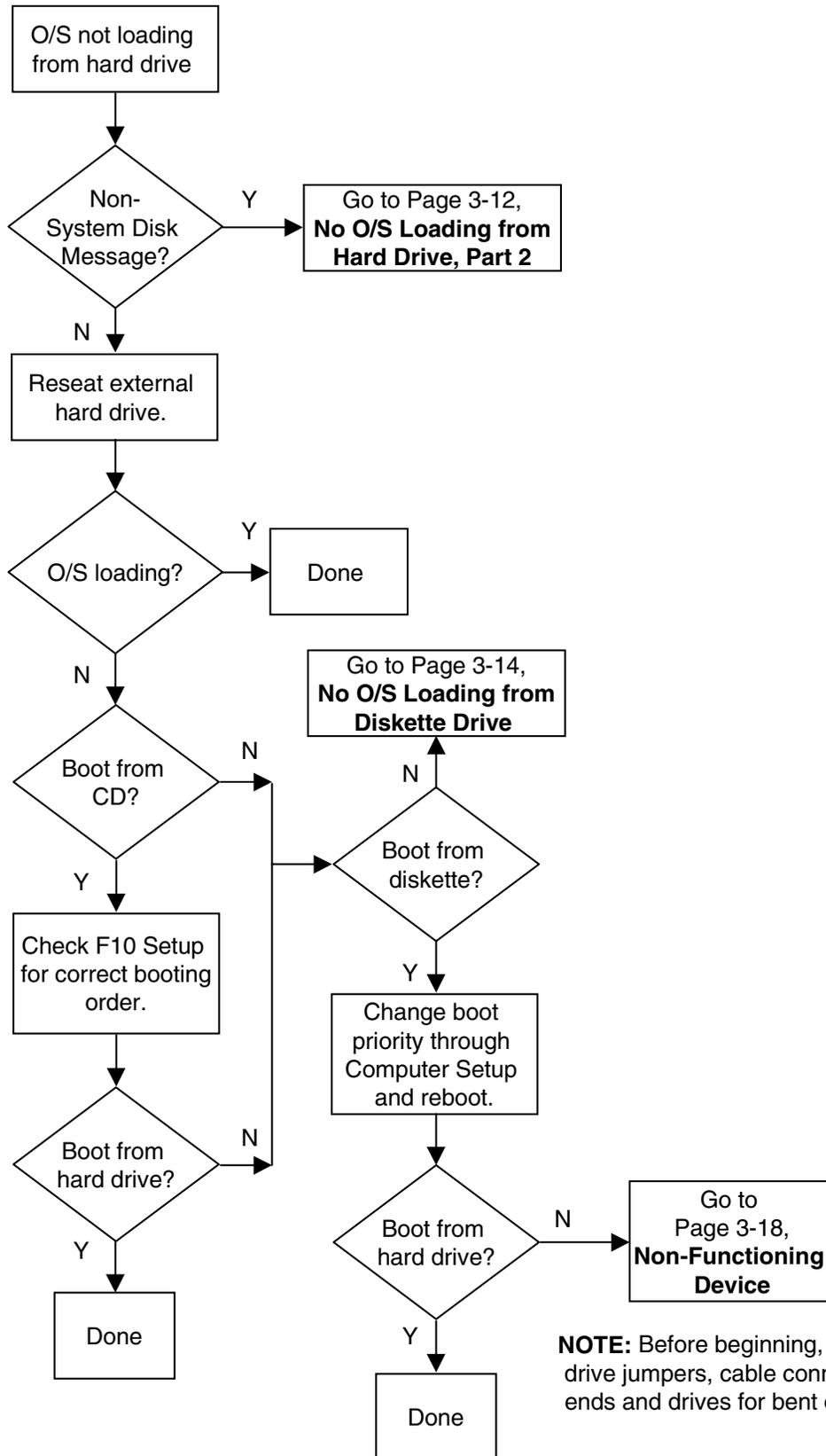
**NOTE:** Before beginning, always check drive jumpers, cable connections, cable ends and drives for bent or damaged pins.
